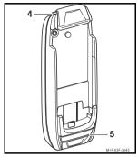
Press the Bluetooth® button (4) for approximately 2 seconds. The LED (5) flashes rapidly. The mobile phone cradle switches to Discovery Mode and can be recognised by the mobile phone.
