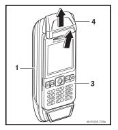
Slide the locking tab (4) upwards and remove the mobile phone (3) from the cradle (1).
