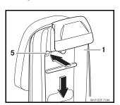
Press the release button (5), slide the cradle (1) downwards and remove.
