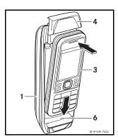
Place the mobile phone (3) on the contact surface (6) and press lightly above the display to engage it into place in the cradle (1).
