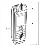
Slide the locking tab (4) upwards and remove the mobile phone (3) from the cradle (1) as shown in the illustration.
