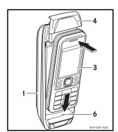
Place the mobile phone (3) on the contact surface (6) and press lightly above the display to engage it into place in the cradle (1).
