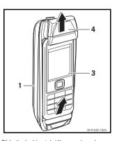
Slide the locking tab (4) upwards and remove the mobile phone (3) from the cradle (1) as shown in the illustration.
