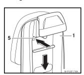
Press the release button (5), slide the cradle (1) downwards and remove.
