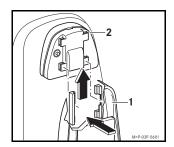
1. Slide the cradle (1) onto the contact plate (2) until it audibly engages.
