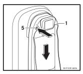
2. Press the release button (5), slide the cradle (1) downwards and remove.
