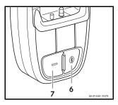
Press the Bluetooth<sup>®</sup> button (6) for approximately 2 seconds. The LED (7) flashes rapidly. The cradle is visible to searching devices for approx. 2 minutes and can be detected by the mobile phone.
