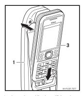
1. Insert the mobile phone (3) into the cradle (1) as shown.
