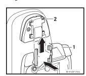
Slide the cradle (1) onto the contact plate (2) until it audibly engages.
