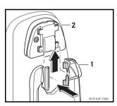
Press the mobile phone cradle (1) into the catches of the bracket (2) and push it upwards until it audibly engages.
