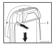
2. Press the release button (7), slide the cradle (1) downwards and remove.
