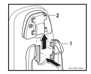
Press the mobile phone cradle (1) into the catches of the bracket (2) and push it upwards until it audibly engages.
