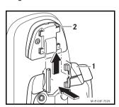
Slide the cradle (1) onto the contact plate (2) until it audibly engages.
