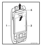
Slide the locking tab (6) upwards and remove the mobile phone (3) from the cradle (1).
