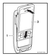
Insert the mobile phone (3) into the cradle (1) as shown.
