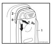
2. Press the release button (6), slide the cradle (1) downwards and remove it from the bracket (2).
