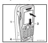
Press the mobile telephone (3) onto the connector (4) and engage the upper part in the cradle (1) as shown. The mobile telephone changes to hands-free mode and a message appears in the display of the mobile telephone (please refer to the operating instructions of the mobile telephone). If this is not the case, remove the mobile telephone and re-insert if.
