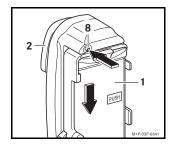
2. Press the release button (8), slide the cradle (1) downwards and remove it from the bracket (2).
