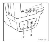
2. Press the Bluetooth<sup>®</sup> button (6) for approx. 2 seconds. The LED (7) flashes rapidly. The mobile phone cradle switches to Discovery Mode and can be recognised by the mobile phone. MB V3 Cradle appears on the mobile phone display to indicate the mobile phone cradle.
