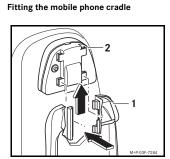
Press the mobile phone cradle (1) into the catches of the bracket (2) and push it upwards until it audibly engages.
