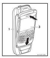
Insert mobile phone (3) into the cradle (1) as shown so it engages into place.
