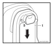
1. Press the release button (5), slide the cradle (1) downwards and remove.
