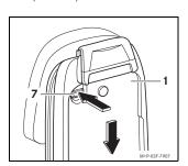
2. Press the release button (7), slide the cradle (1) downwards and remove.
