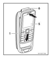
Switch on the mobile phone (5) and insert it into the cradle (1) as shown.
