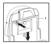
Press the release button (7), slide the cradle (1) downwards and remove
