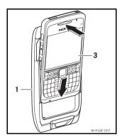
Insert the mobile phone (3) into the cradle (1) as shown.
