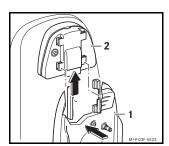
Press the cradle (1) into the catches on the pre-installed retainer (2), keep the cradle (1) pressed and slide it upwards until it clicks into place.
