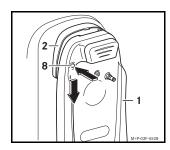
2. Press and hold the release button (8). Slide the cradle (1) downwards and remove it from the pre-installed retainer (2).
