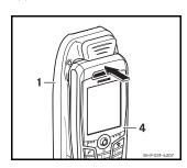
2. Press the upper part of the mobile telephone (4) into the cradle (1) until the mobile telephone (4) engages in the cradle (1).
