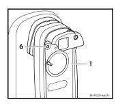
Press the release button (6) with a pointed object, slide the cradle (1) downwards and remove.
