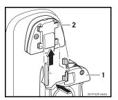
Press the cradle (1) into the catches of the pre-installed bracket (2) and push it upwards until it audibly engages.
