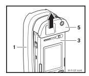
Slide the locking tab (5) upwards and pull the mobile telephone (3) out of the cradle (1).
