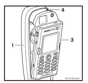
Insert the mobile telephone (3) into the cradle (1) as shown.
