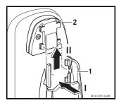
1. Press the cradle (1) into the retainers on the existing mounting (2), keep the cradle pressed and slide it upwards until it clicks into place.
