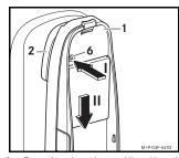
2. Press the release button (6) and keep it pressed. Slide the cradle (1) downwards and remove it from the existing mounting (2).
