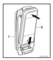
1. Place the mobile phone (3) onto the plug connector of the cradle (1) and guide it into the cradle using light pressure above the display until it audibly engages into
