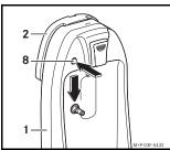
Press the release button (8) and keep it depressed. Slide the mobile phone cradle (1) downwards and remove it from the existing
