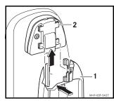
1. Press the mobile phone cradle (1) into the retainers on the existing mounting bracket (2), hold it in place and slide the cradle (1) upwards until it clicks into place.
