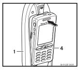
3. Press the upper end of the mobile phone (4) into the cradle (1) until the mobile phone (4) clicks into place in the cradle (1).
