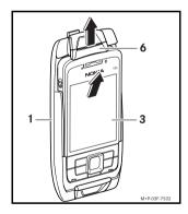
Slide the locking tab (6) upwards and remove the mobile phone (3) from the cradle (1).
