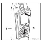
2. Insert the mobile phone (3) into the bracket (1) as illustrated.
