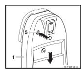
Press the release button (5), push the bracket (1) downwards and detach.
