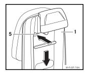
Press the release button (5), slide the cradle (1) downwards and remove.
