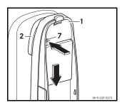
Press and hold the release button (7). Slide the cradle (1) downwards and remove it from the pre-installed retainer (2).
