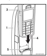
Slide the mobile telephone (3) from above into the cradle (1) so that the catches (4) are pressed apart. Push the mobile telephone (3) onto the plug connector (5), and then press the upper section of the mobile telephone (3) downwards and at an angle into the cradle (1) until the mobile telephone (3) is engaged.
