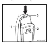
Press the release button (6), and take the mobile telephone (3) out of the cradle (1).
