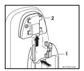
Press the bracket (1) into the catches of the pre-fitted retainer (2) and push it upwards until it audibly engages.
