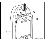
Push the release (5) upwards and pull the mobile phone (3) out of the bracket (1).
