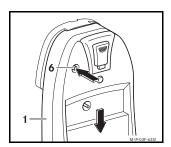
2. Press the release button (6), push the bracket (1) downwards and detach.
