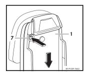
2. Press the release button (7), slide the cradle (1) downwards and remove.
