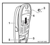
3. Press the upper end of the mobile phone (4) into the cradle (1) until the sides of the mobile phone (4) engage in the cradle (1).
