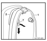
2. Press the release button (7) and keep it pressed. Slide the mobile phone cradle (1) downwards and remove it from the existing mounting bracket (2).
