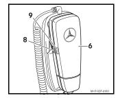
3. Press and hold the thumbwheel (8) on the receiver (6) for approx. 3 seconds without turning it. The LED (9) flashes rapidly. WAIT... appears in the audio system dis play.
