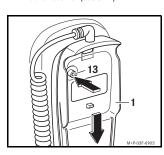
2. Press the release button (13), slide the telephone module (1) downwards and remove.
