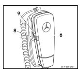
2. Briefly press the thumbwheel (8) on the receiver (6) without turning it. The LED (9) flashes slowly and a message appears in the COMAND or audio system display indicating that the telephone is being activated. The telephone module always searches for and connects the previously paired mobile phone.
