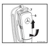
1. Insert the top of the receiver (6) into the retaining lug (7) and press the bottom until it engages into place.
