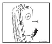
1. Lift the bottom of the receiver (6) and remove it.
