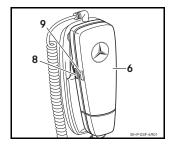
Press and hold the thumbwheel (8) on the receiver (6) for approx. 3 seconds without turning it. The LED (9) flashes rapidly. A message appears in the COMAND display indicating that the telephone is being activated.
