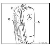
3. Press and hold the thumbwheel (8) on the receiver (6) for approx. 3 seconds without turning it. The LED (9) flashes rapidly. A message appears in COMAND or the audio system display indicating that the telephone is being activated.
