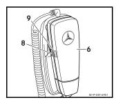
3. Press and hold the thumbwheel (8) on the receiver (6) for approx. 3 seconds without turning it. The LED (9) flashes rapidly.  ${\tt WAIT}\ldots$  appears in the multi-function display.
