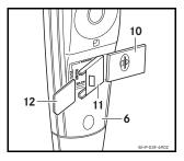
2. Open the cover (10) below the receiver's earpiece (6), slide the SIM card holder (11) towards the right and flip it up.
