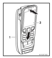
Switch on the mobile phone (3) and insert it into the cradle (1) as shown.
