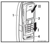
1. First of all, slide the bottom of the mobile phone (3) onto the connector (4) and then press the top of the mobile phone downwards at an angle into the cradle (1) until the mobile phone (3) clicks into place.
