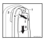
2. Press the release button (6) and keep it pressed. Slide the cradle (1) downwards and remove it from the existing mounting (2).
