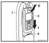
1. First of all, slide the bottom of the mobile phone (3) onto the connector (4) and then press the top of the mobile phone downwards at an angle into the cradle (1) until the mobile phone (3) clicks into place.
