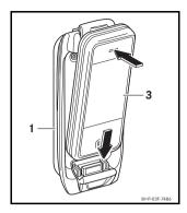
1. Place the mobile phone (3) onto the plug connector of the cradle (1) and guide it into the cradle using light pressure above the display until it audibly engages into place.
