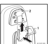
1. Slide the cradle (1) onto the contact plate (2) until it audibly engages.
