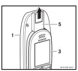
Slide the locking tab (5) upwards and remove the mobile telephone (3) from the cradle (1).
