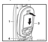
Press the mobile telephone (3) onto the connector (4) and engage the upper part in the cradle (1) as shown.
