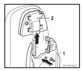
Press the cradle (1) into the catches of the bracket (2) and push it upwards until it audibly engages.
