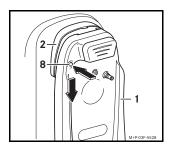
Press and hold the release button (8). Slide the bracket (1) downwards and remove it from the pre-installed retainer (2).
