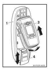
Slide the catch (4) downwards, place the mobile phone (3) into the cradle (1) as shown and slide the catch (4) upwards.
