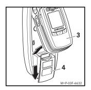
Slide the catch (4) downwards and remove the mobile phone (3) as shown.
