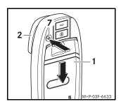
2. Press the release button (7), slide the cradle (1) downwards and remove it from the bracket (2).
