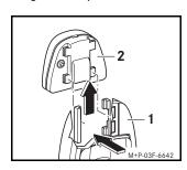
Press the cradle (1) into the catches of the bracket (2) and push it upwards until it audibly engages.
